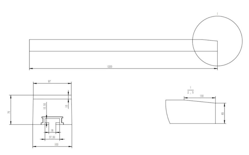
The impact bar is a component or structure designed to absorb and mitigate the force of an impact. It is commonly used in various applications to protect against damage or to enhance safety for conveyor system, improves the efficiency of the conveyor system and reduces maintenance cost. Impact Bar is made of three parts
